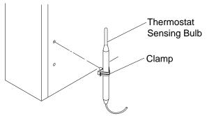
Figure 5 - Attaching Thermostat Sensing Bulb
